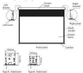
A-Type ceiling cut out dimension: cut out length Lt = Screen Total length – 26mm; cut out width 150mm, height ≥ 160mm;
