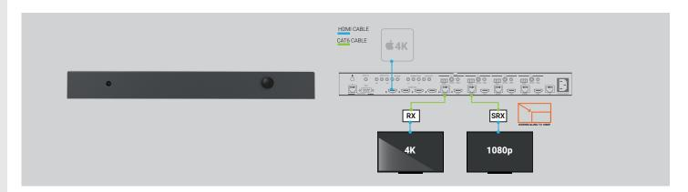
Delivering end-to-end 4K/60 Hz switching and scaling, including support for HDCP 2.2 - the MHUB SRX scaling display receiver is a simple way to overcome the real-world problem of utilising a mix of UHD/4K and 1080p TVs, or projectors within the same centralised AV system, whilst ensuring every connected display always operates at best capability.
