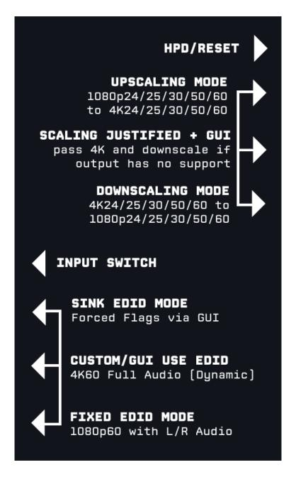
A sticker is available on the back of the unit to remind you the basic configuration options available from the physical button and slide switches.
