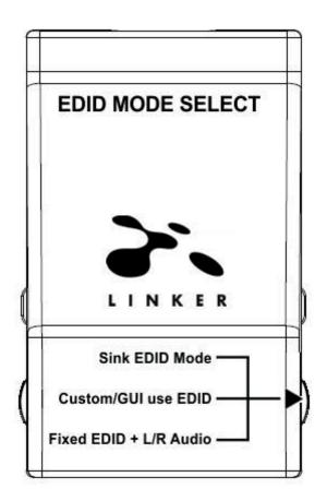
EDID slide switch has 3 positions. Switch should be set to middle position to allow control via Windows PC USB GUI.
