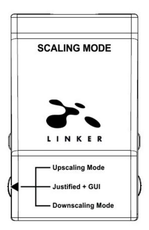
Scaling Mode slide switch has 3 positions.
