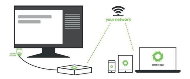
The requirements for an operational system are straightforward. The display is connected via HDMI video cable to a Solstice Pod or Solstice Windows host PC. The Solstice host is attached to the WiFi/Ethernet network participants will user to connect and share to the display. Then, users on the network can follow on-screen instructions to get the Solstice app and connect to the display.
