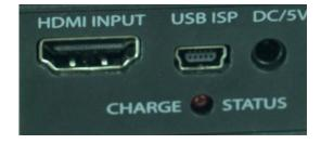
n. HDMI Input connector – connect to any source or repeater output via HDMI cable.
