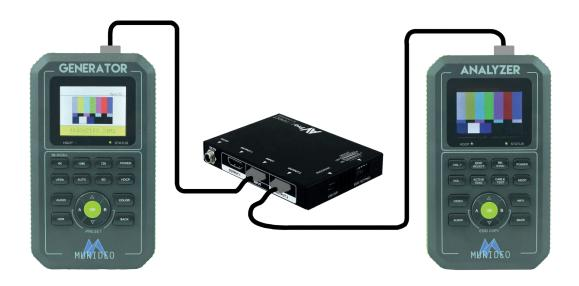
How to Test a Repeater (a repeater is any HDMI device that receives an input signal and retransmits that same signal to a downstream sink or display device; like a matrix, a switch, an AV receiver or distribution amplifier)
