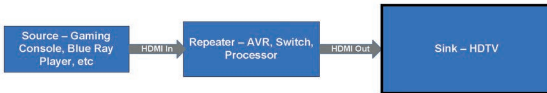
Connection Diagram Fresco SIX-G
