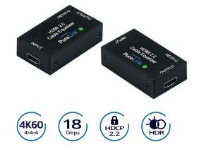
The **HE101-U** Signal Equalizer provides a convenient installation solution for extending and amplifying high-bandwidth HDMI 2.0 signals using standard HDMI cables in a home or office environment.
