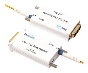
The OLC III Tx/Rx DVI over One Fiber Extension System provides long range extension of DVI to distances up to 980 ft. (300 m.) over a single strand, LC-terminated fiber optic cable. Real-time EDID programming provides fast integration and compatibility between input and output devices.
