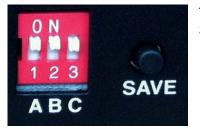
Turn ON switch 2. Select settings for switch 3, then press SAVE to store internal EDID data.
