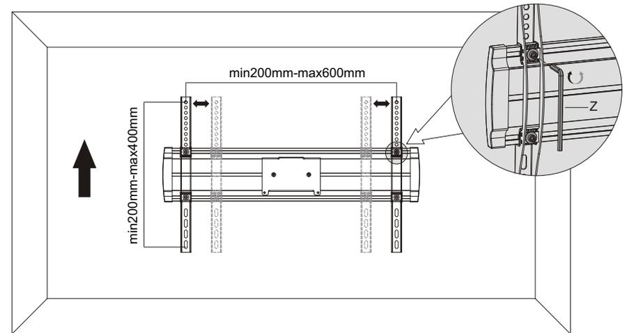
Adjust the adapter brackets to fit the hole pattern of your display. Then tighten all screws with an allen key. **NOTE:** Verify the proper alignment of all holes.
