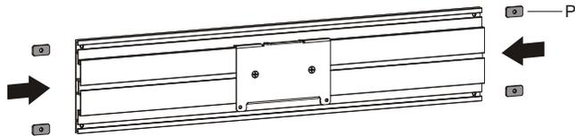
Insert the washers into the back of universal plate along the plate rails.
