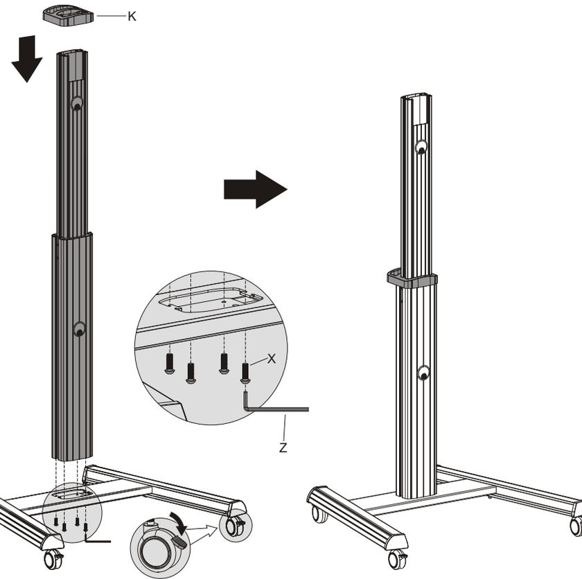
Attach the column to the base using the screws. Tighten all screws using an allen key.
