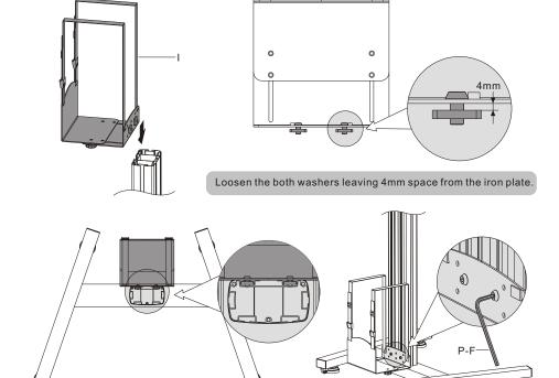
Insert the host machine rack to the desired position along the column slots, Tighten all screws with an Allen key to secure.
