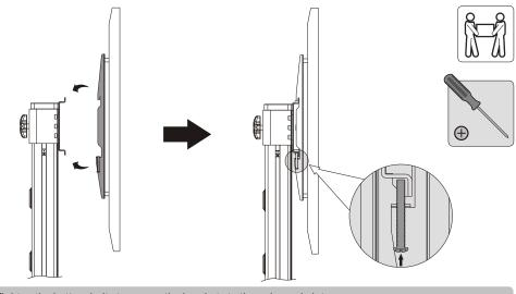
Tighten the bottom bolts to secure the brackets to the universal plates.
