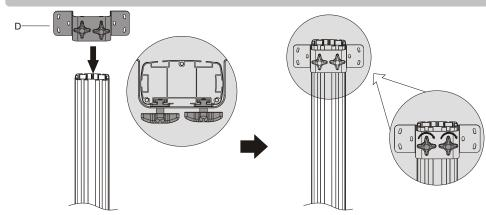
Insert the fixing piece to the desired position along the back slots of the column. Level the fixing piece and tighten both knobs.
