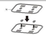
Remove the two caps from the camera shelf, Attach the camera shelf to the support rods using four screws and tighten all screws to secure it and then reattach the caps to the camera shelf.
