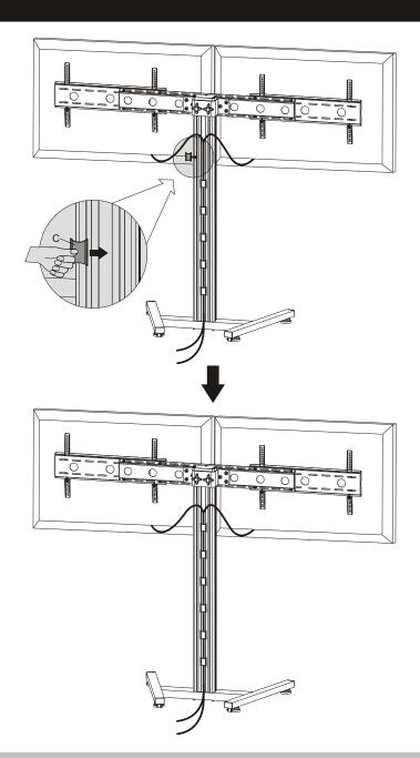
• Use the cable clips for routing cables.
