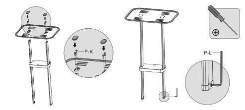
Loosen the screws(but don't remove) on the bottom of support rods.
