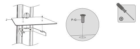
Attach the iron shelf to the shelf support using three screws, thighten them with a proper screwdriver.
