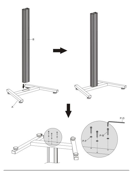
Attach the column to the base using the appropriate screws and washers, Then tighten all screws to secure them.
