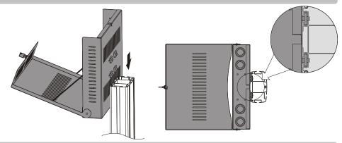
Insert the laptop box to the desired position along the column slots. Then tigten all screws to secure.
