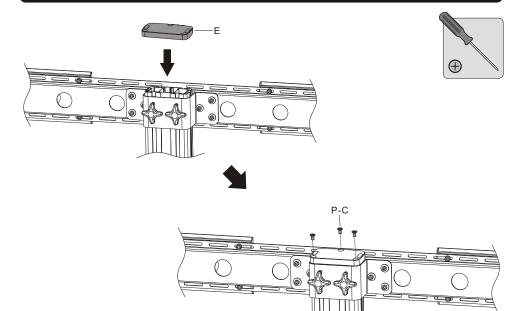
Use three screws to fasten the top cover.
