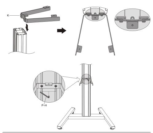
Insert the shelf support to the desired position along the front slots of the column. Tighten the two screws to secure it.
