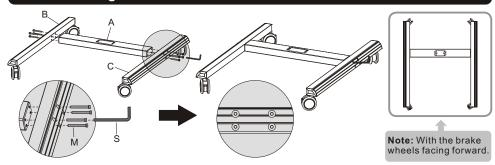
Attach the left and right base to the middle base using the appropriate screws. Tighten all screws with an Allen key.
