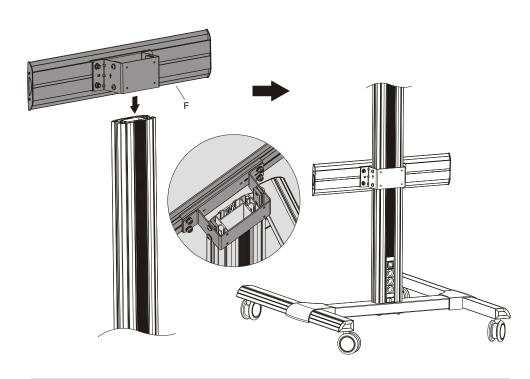
Insert the universal plates to the column along the column rails respectively. **NOTE:** With the arrow pointing upward.
