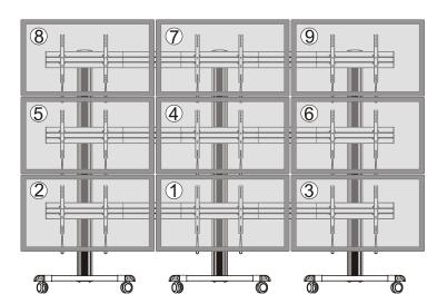
Note: The displays are installed by the numerical order given.
