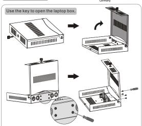
Loosen all screws in order to separate the connecting piece from the laptop box.
